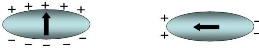
Fig. 4: The shape anisotropy of a homogeneously magnetized, elongated particle is a magnetostatic effect: An alignment of the magnetization with the long axis (sketch on the right) minimizes the magnetostatic surface charges. The configuration therefore has a lower magnetostatic energy than a transversal orientation (left), thereby giving rise to a shape-dependent preferential direction (“easy axis”) of the magnetization.
